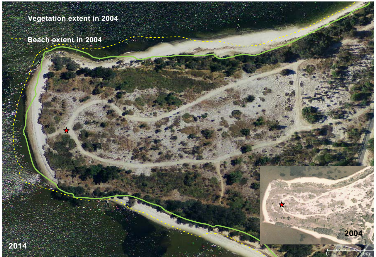
Figure 4 Rate of erosion at the spit end between January 2004 and January 2014 (Image source: Landgate Map Viewer: https://www.landgate.wa.gov.au/bmvf/app/mapviewer/ )
